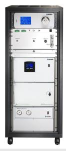
The DCS system is a complete rack-mounted calibration station capable of producing a flow of air (or nitrogen) at a pre-specified range of dew-point temperatures from a minimum of -100 °C (-148 °F) to a maximum of +20 °C (+68 °F).
